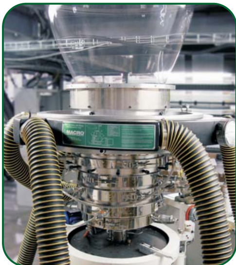
Monolayer die and D10 air ring producing an evenly gauged, perfectly cooled bubble
