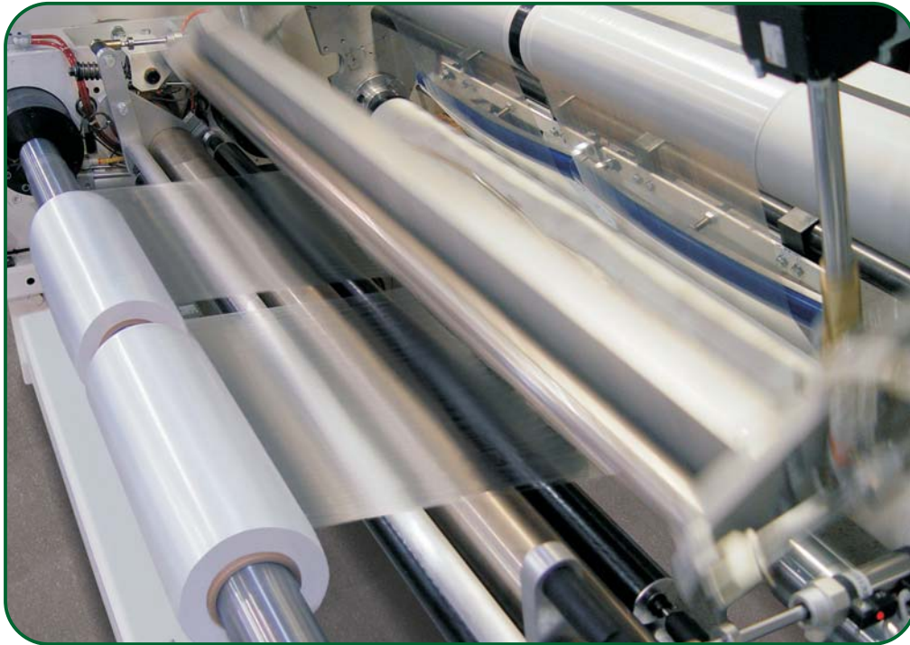
Automatic cut and roll transfer of soft prestretch film rolls on Macro's BPS Line
