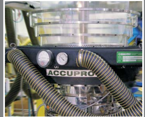
Blown Film Die Outfitted with an ACCUPRO Die-Based Gauge Control System
