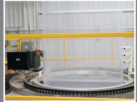
Rotating Scanner consisting of a Gamma Backscatter Sensor mounted to a Telescoping Probe Positioner 2
