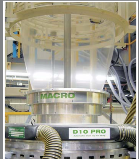
Blown Film Line Outfitted with the D10PRO Automatic Dual Lip Air Ring
