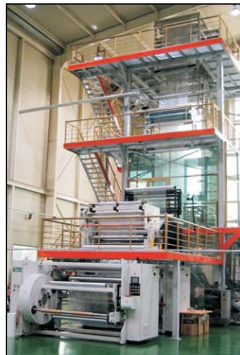
7-Layer BXL Barrier Blown Film Line
