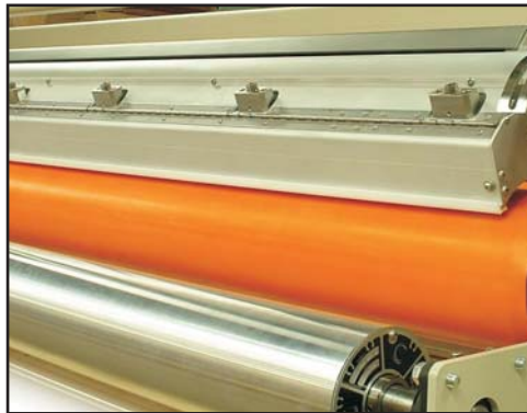
Corona Treater (Courtesy of Enercon)
